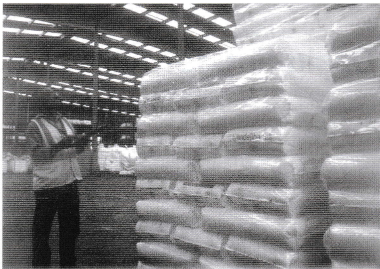
LyondellBasell says shipping sack and stretch hooder applications can be down-gauged in part by using its Starflex mLLDPE.
